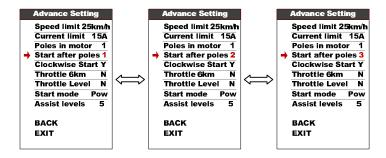
**8.16 Clockwise start**: This parameter represent speed sensor turn direction, default value is Y (forward).
