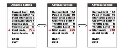
**8.20 Assist levels**: This parameter can customize assist levels, options are 3/5/9/UBE, UBE represent factory default settings.
