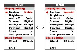
**8.2 Brightness**: Press Up / Down button to change the brightness of the backlight, is darkness, is brightness
