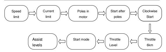
**8.12 Speed limit**: Press UP/DOWN will change speed limit, range 10km/h~45km/h. Default value is 25km/h.
