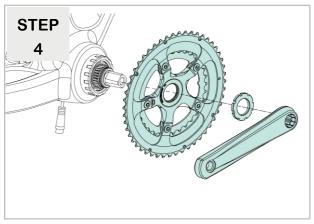
Install the chainwheel, groove nut and cranks.
