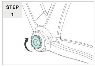
Insert and tighten the left side bottom bracket bowl cup with torque to 35 Nm.
