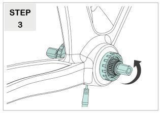
Insert and tighten the bracket bowl cup of the left side bottom with torque to 35 Nm.  $\,$
