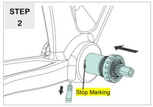
Insert the sensor from the left side and pull the cable from the bottom bracket's bottom hole.
